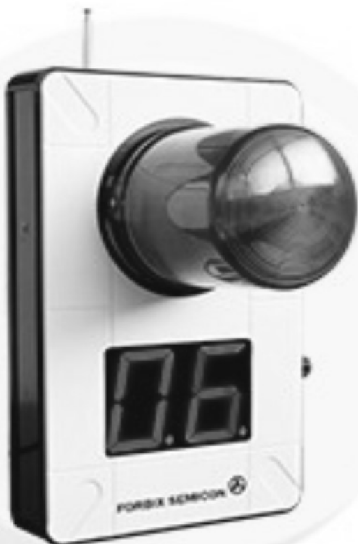
Revolving light with display at the guard room
